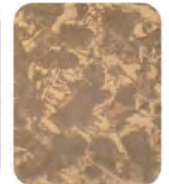
100× 珠光体轧 辊金相组织 100× Pearlitic roll metallographic structure
