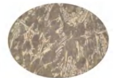
100× 中镍球无轧辊 金相组织 100× Medium nickel ductile indefinite chill cast roll metallographic structure
